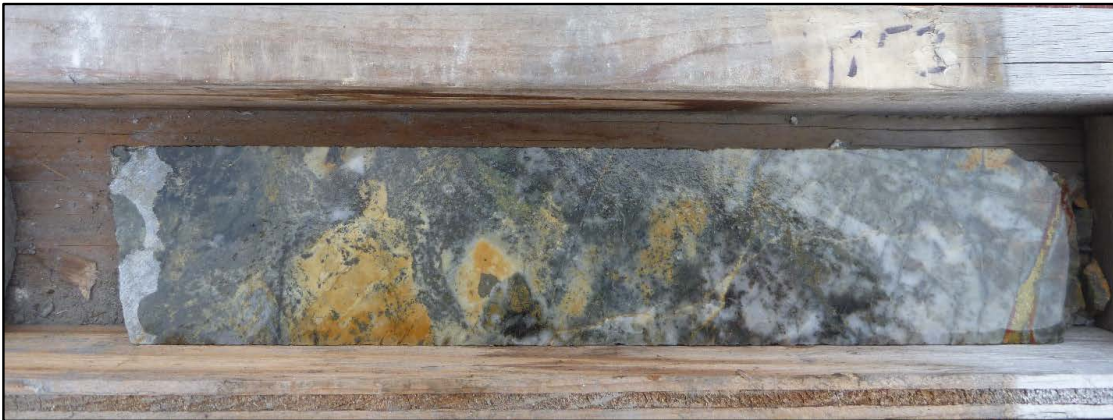
Figure 25: Section of Sample V944306, re-sample of JN19021-045, 253.0 - 253.84m (original: 3.50 g/t Au)
