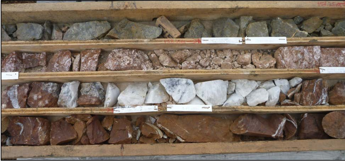
Figure 20: Sample V944301: re-sample of JN11009-129, 159.05 - 159.55 m (3rd row from top, original: 9.77 g/t Au).
