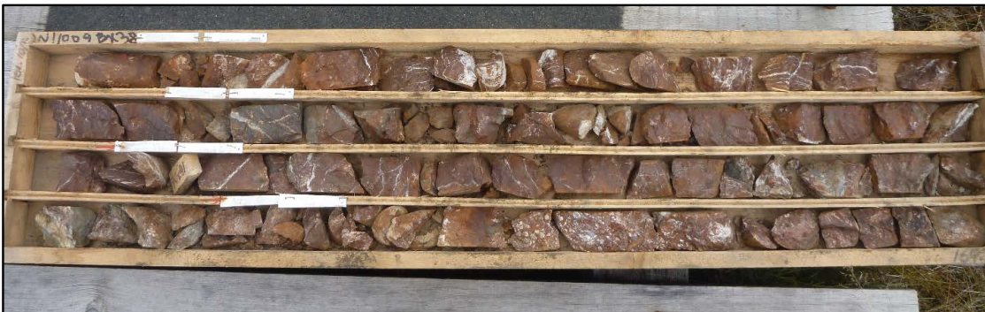
Figure 21: Sample V944302: re-sample of JN11009-133, 162.20m - 163.00m (2nd row from top, original: 3.48 g/t Au)
