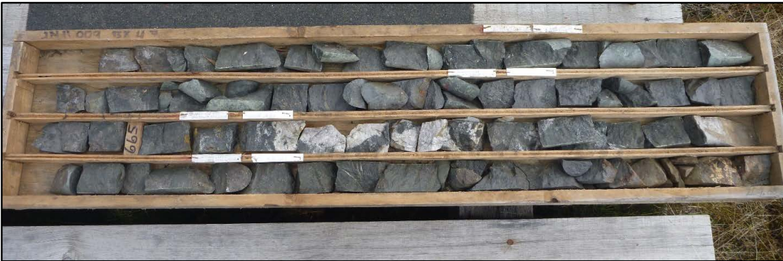
Figure 23: Sample V944304: re-sample of JN11009-175, from 202.80 m - 203.85 m (3 rd row from top, original: 12.45 g/t Au)
