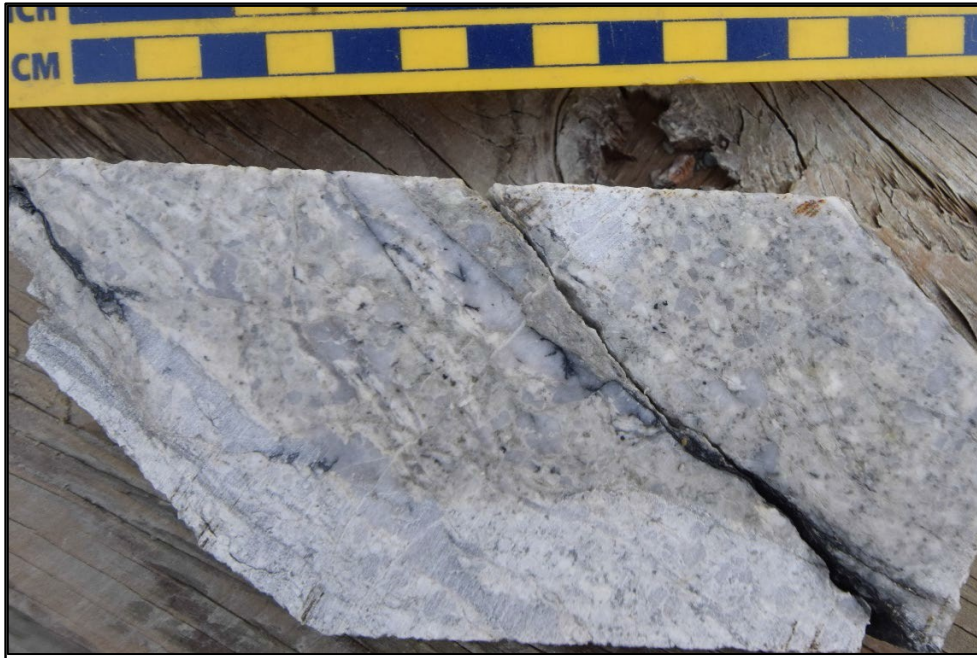
Figure 46: Molybdenite along margins of sheeted veins within Justin intrusion. DDH JN19039, 55.1m (Bates, 2020)
