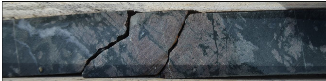
Figure 42: Prograde skarn, Yusezyu Formation. Coarse crystalline red-pink garnets. DDH JN19020, 174.8 m (Bates, 2020)
